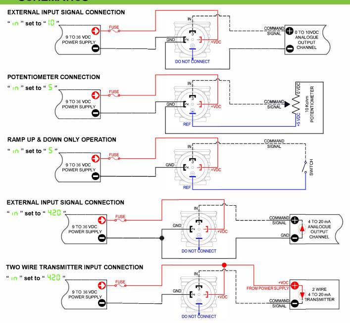
**PLEASE NOTE:** For "0 to 5 VDC" & "0 to 10 VDC" command input drivers, it is recommended to use independent negative conductors for power supply and analogue output channel (PLC/PC) to maintain command signal accuracy due to voltage drop on long cable runs.
