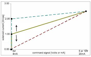
rup: RAMP UP. Time for Output to Increase from min to max, 0.0 to 99.5 [SEC]
